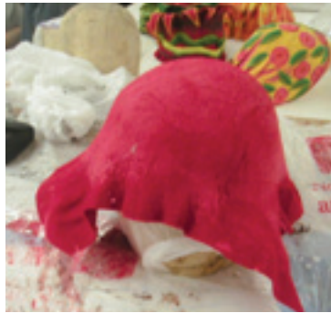
Figure D2: Felt shaped over former
