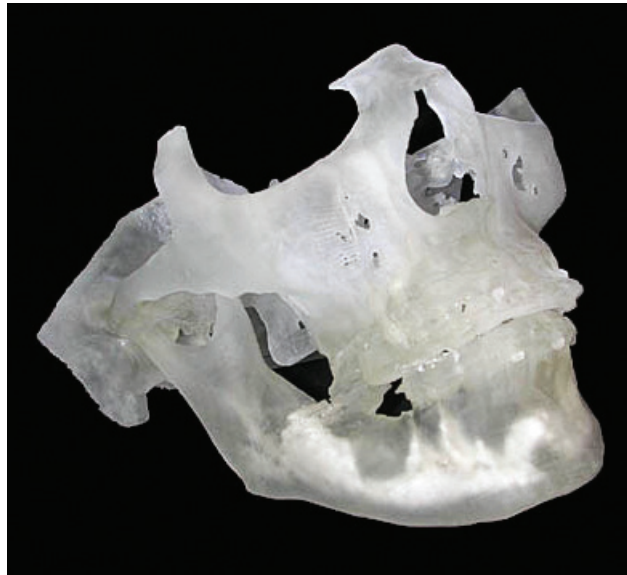
Figure C2: Physical prototype made using stereo lithography
